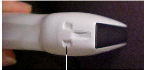
Alignment Depressions on the 12L5 Transducer
