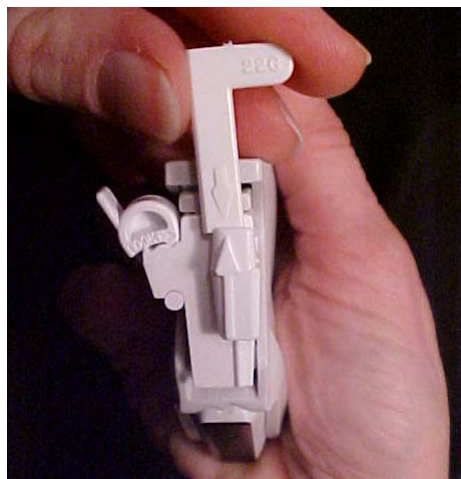
Aligning the Needle Guide Clip
