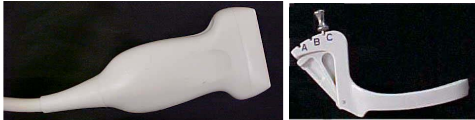
12L5 Transducer (Left) and Bracket (Right)
