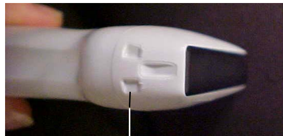
Alignment Depressions on the 10L5 Transducer
